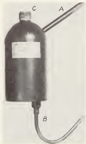
17-31. A high pressure side float refrigerant control. A. Inlet; B. Outlet; C. Purging and service valve attachment fitting. (Aminco Refrigeration Products)
